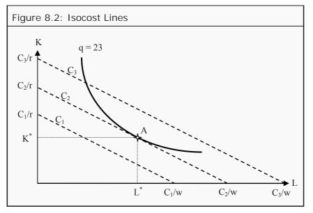
Just as we did in consumer theory, we can give a mathematical formulation of the result. At the point of tangency, the isoquant and the isocost line must have the same slope. The slope of the isocost line is -w/r and the slope of the isoquant is the marginal rate of technical substitution, MRTS (see Section 7.4). At the point of tangency, we must then have that
