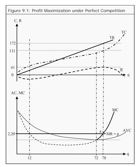
In the lower part of the diagram, we have drawn the **marginal revenue**, MR, the price, p, the **marginal cost**, MC, and the average variable cost, AVC. MR corresponds to the slope of TR, which we argued must be equal to p. In other words, if we sell one more unit of the good, we receive an additional income equal to the price, p. Therefore, MR is equal to p.
